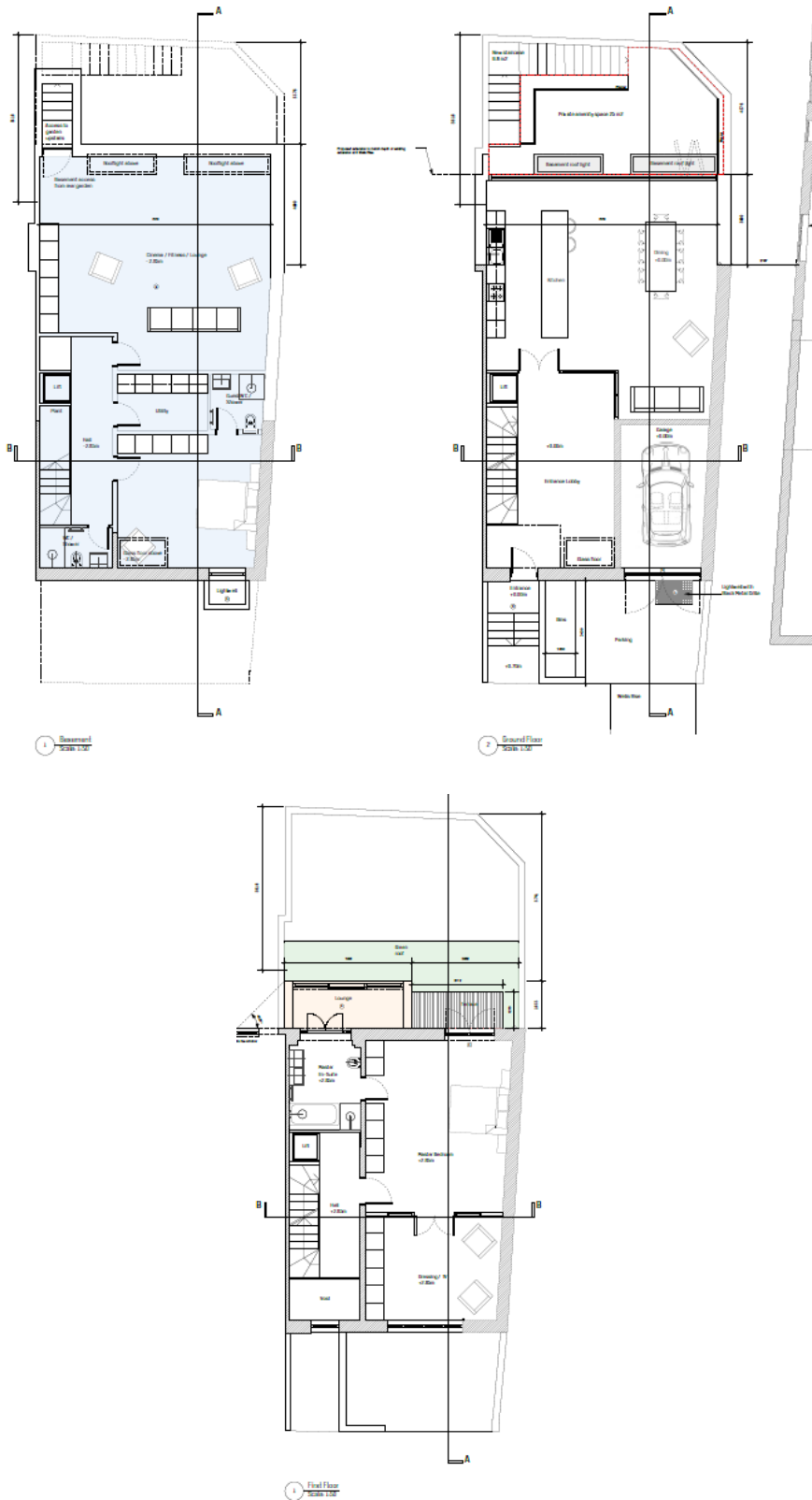
Proposed basement and ground floor plans (top) and proposed first floor plan (bottom).
